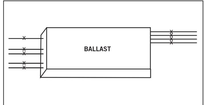
5. From mains, connect input (L) line to all wires coming from sockets on one side of sign and (N) neutral to all wires coming from the sockets on opposite end of the sign.
