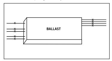
**5.** From mains, connect input (L) line to all wires coming from sockets on one side of sign and (N) neutral to all wires coming from the sockets on opposite end of the sign.
